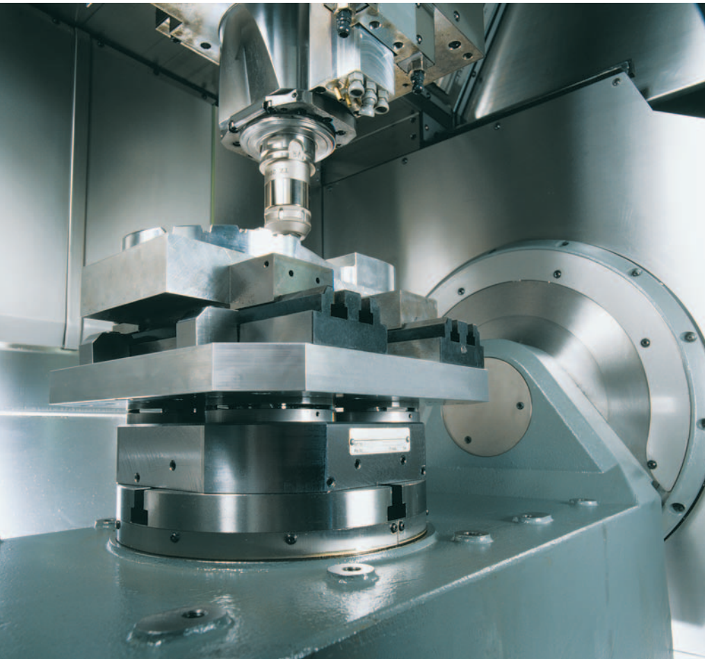
High precision rotary/swivel table with maximum performance capability due to INA/FAG bearing solutions
